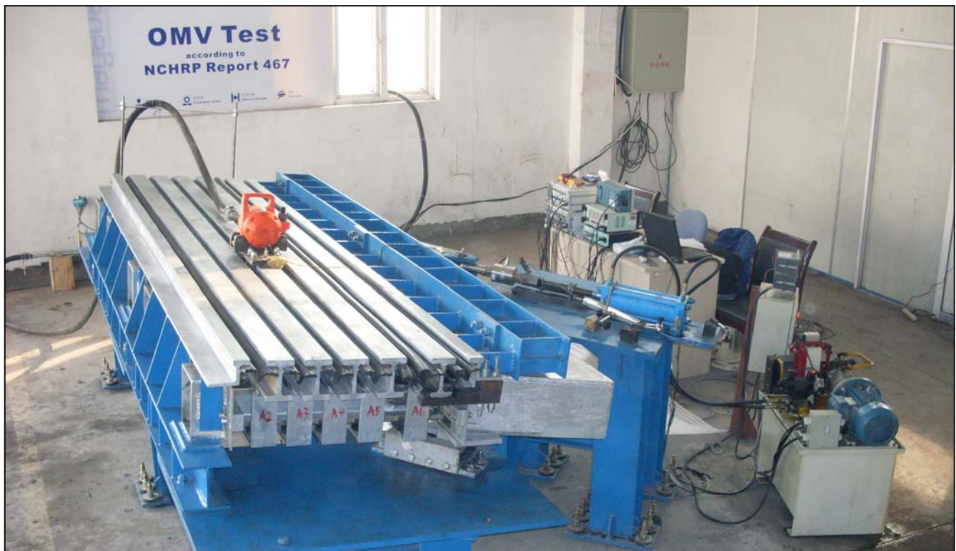
Figure 7. Opening Movement & Vibration (OMV) Test
