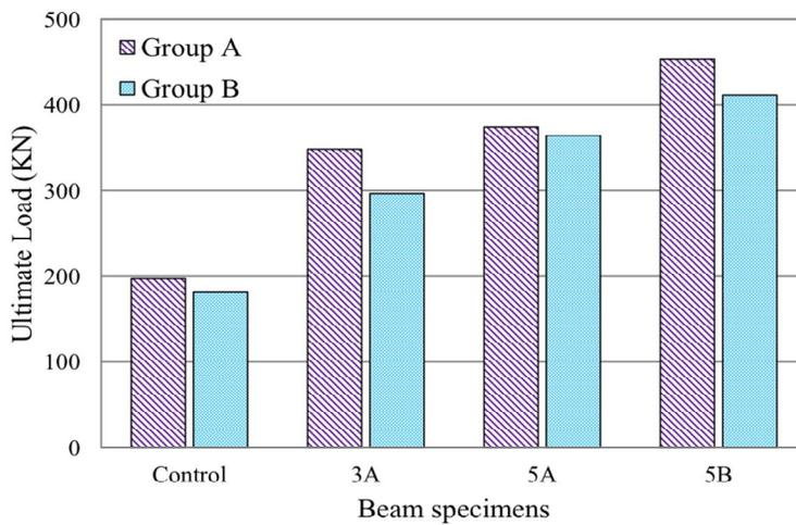
Figure 12. Effect of openings size
