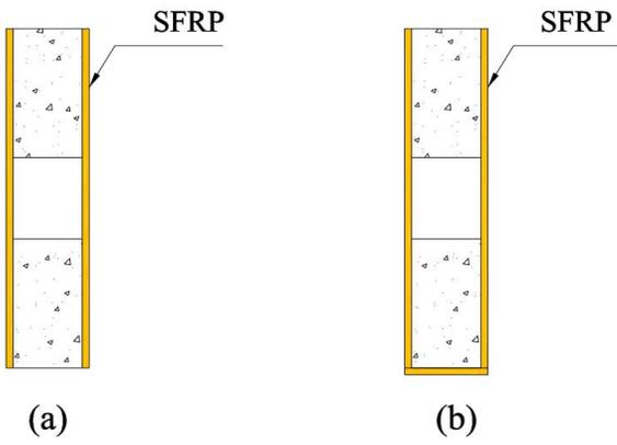
Figure 3. SFRP strengthening configurations; (a) SFRP configuration A, (b) SFRP configuration B
