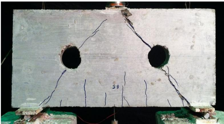
Figure 14. Un-strengthened beam specimen (openings size = 100 mm diameter)
