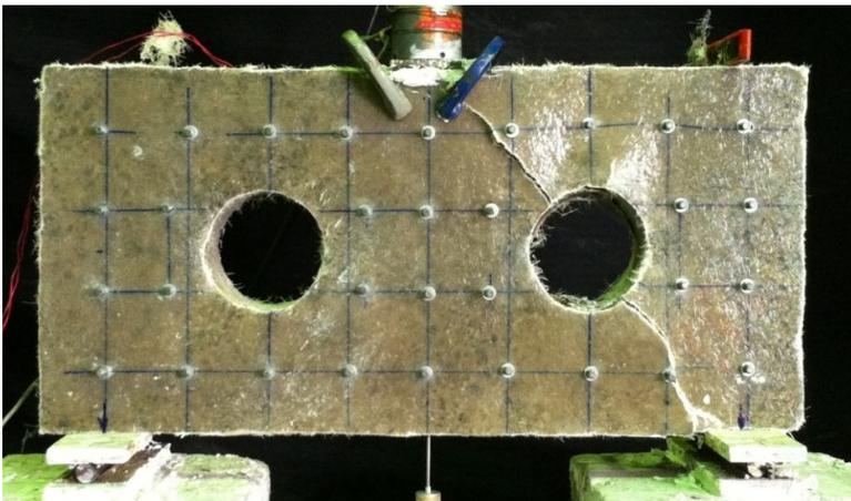
SFRP strengthened beam specimen
