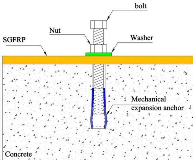
Figure 7. MB anchoring system
