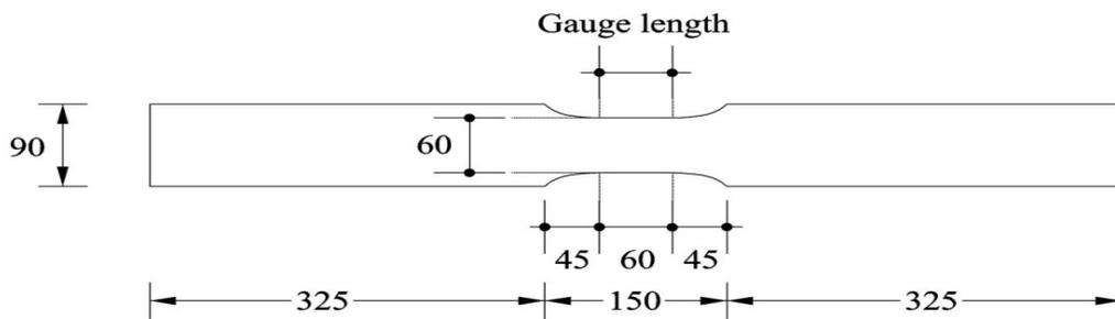
Figure 6. SFRP tensile strip details (unit in mm)
