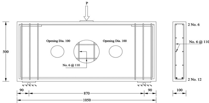
Figure 1. Group A beam details (unit in mm)
