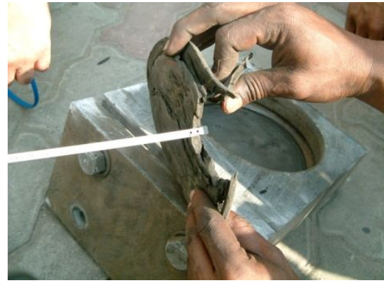
Damaged Hinge bearing
