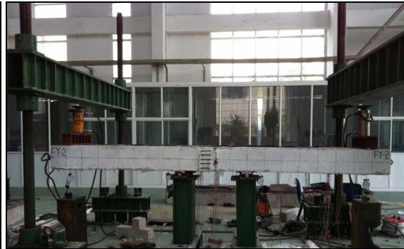
Figure 8. Loading beam with CFRP
