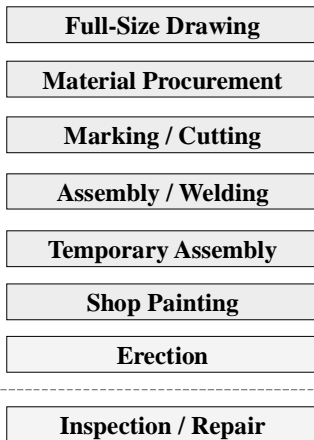
Figure 3. Construction workflow for a steel bridge
