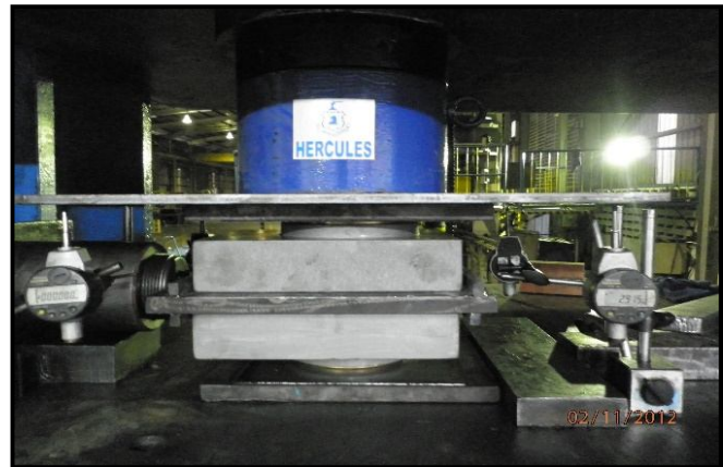
Figure 10. Long term deterioration test on hinge bearing.
