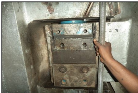
Figure 12. Stress bar clamping system in hinges.
