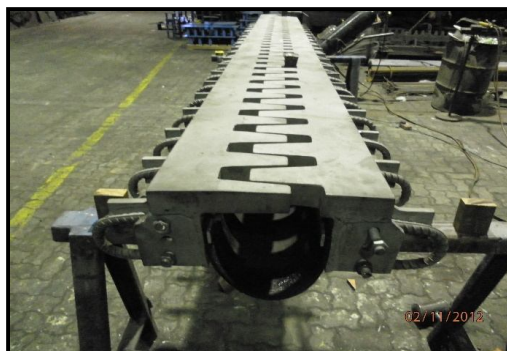
Figure 8. Fabricated expansion joint assembly.
