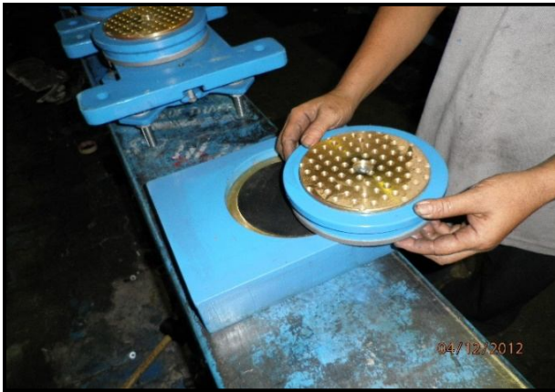
Figure 9. Assembly of permanent hinge bearings.
