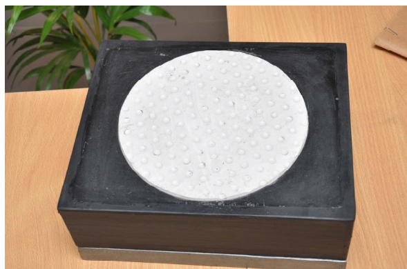
Figure 5. Temporary PTFE topped elastomeric bearing.
