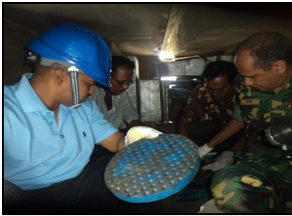
Figure 11. UHMWPE disc in excellent condition after months of service.
