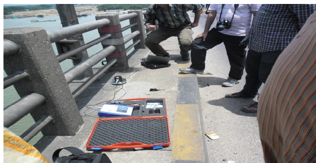
Figure 18. Vibration monitoring in progress.
