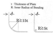
Figure 4. Minimum radius of cold bending
