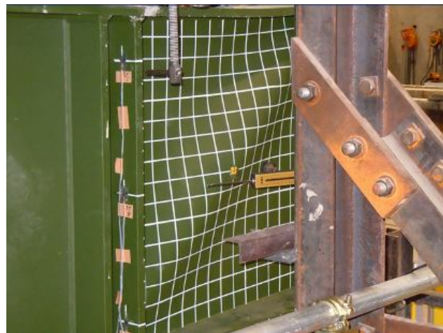
Figure 3. Shear Buckling at Webs
