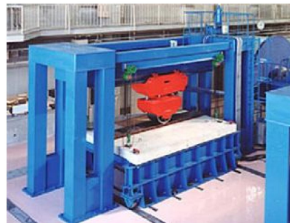
Figure 7. Wheel loading test on RC slab
