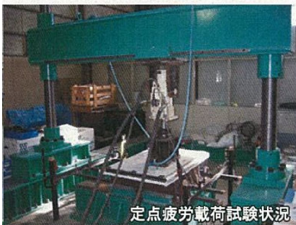
Figure 6. Point loading test on RC slab
