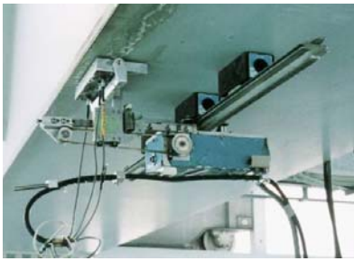
Photo 2. Automated Ultrasonic Testing system
