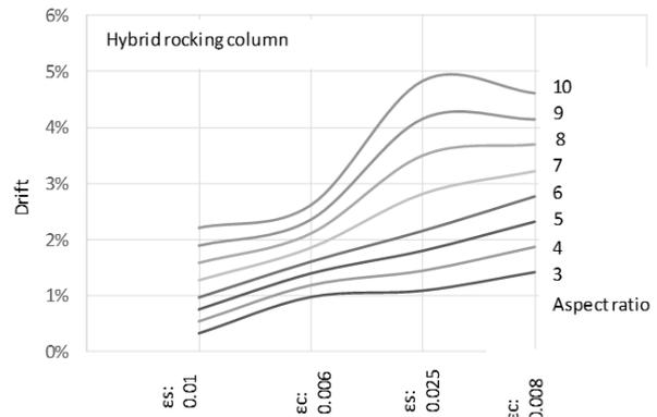
Figure 7. Hybrid rocking column drift vs. damage states.
