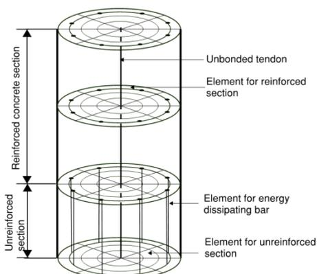
Figure 1. Finite element model of the hybrid rocking column.
