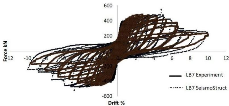
Figure 2. Validation of hybrid rocking column model under static loadings.
