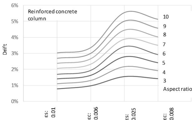
Figure 6. Reinforced column drift vs. damage states.
