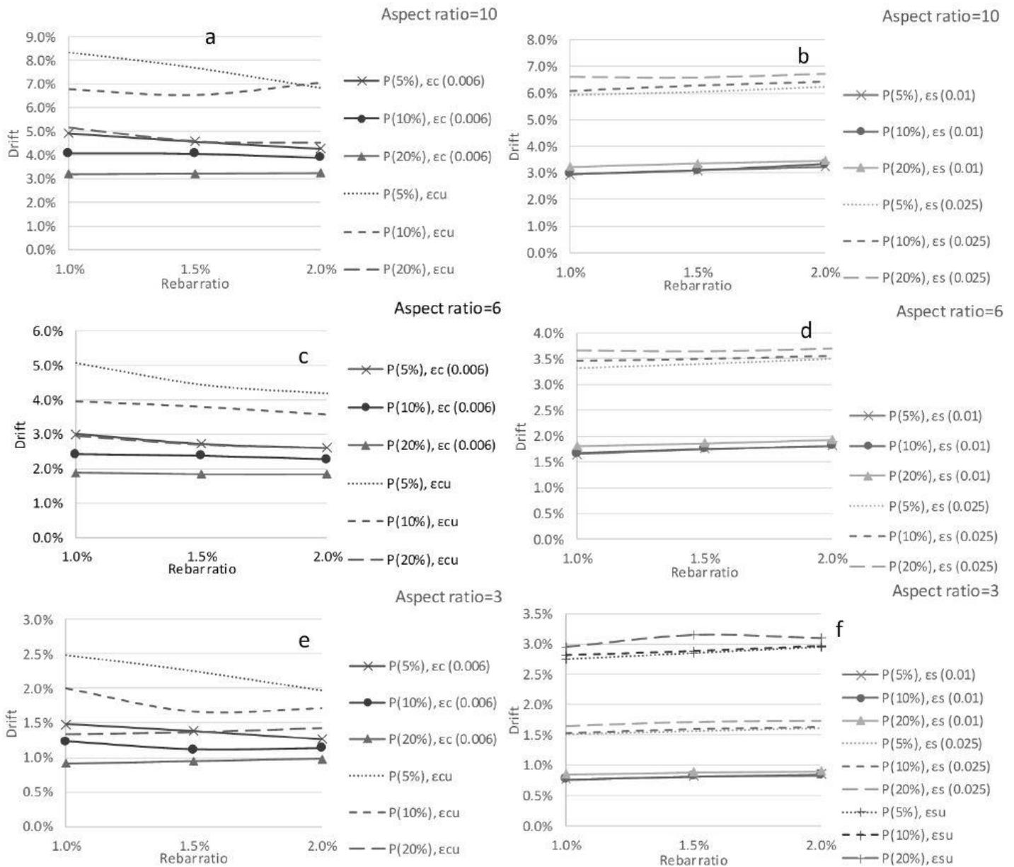
Figure 3. Drift – material strain relations of reinforced concrete columns.
