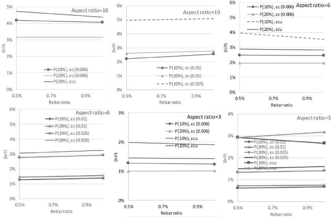
Figure 4. Drift – material strain relations of hybrid rocking columns.
