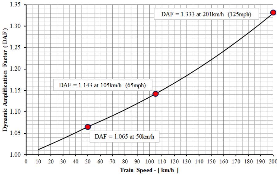
Figure 1. Dynamic amplification factor (DAF) based on Network Rail Code (2006).
