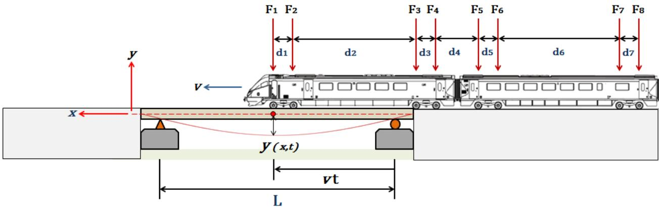
Figure 2. Bridge-rain interaction model.
