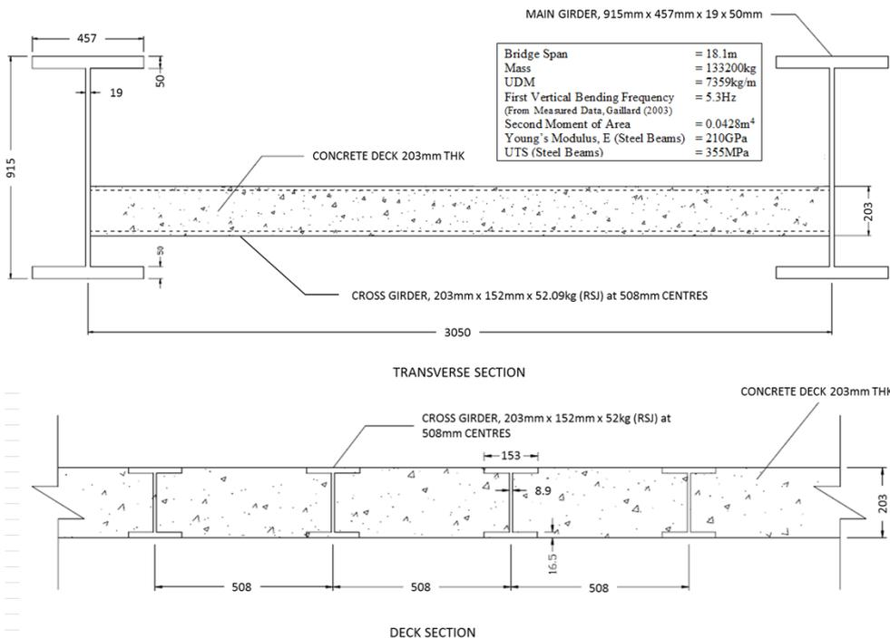
Figure 3. Half-through deck plate girder railway bridge used as case study (Gaillard, 2003).
