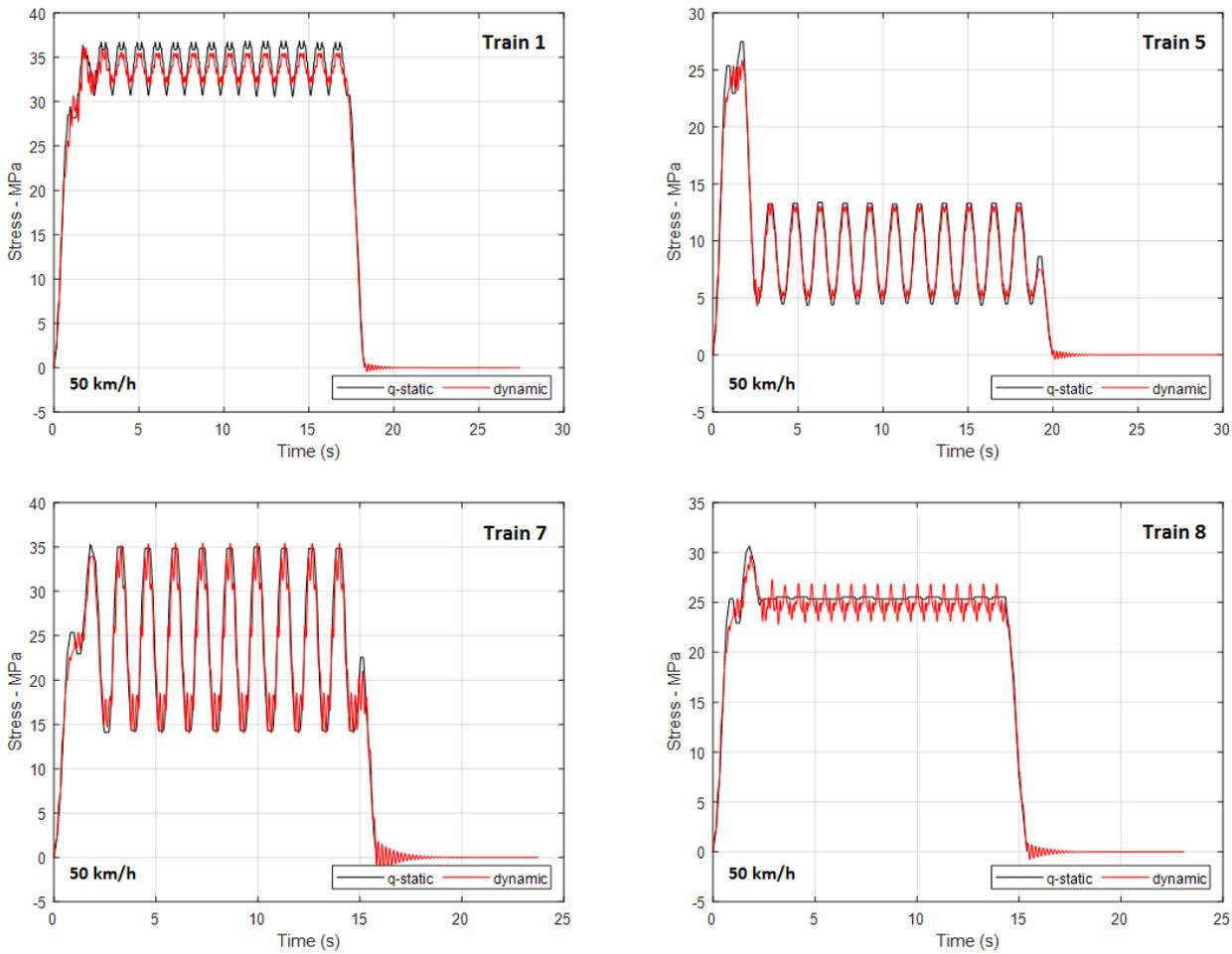
Figure 4. Bridge stress-time response for different trains comparing static versus dynamic analyses.
