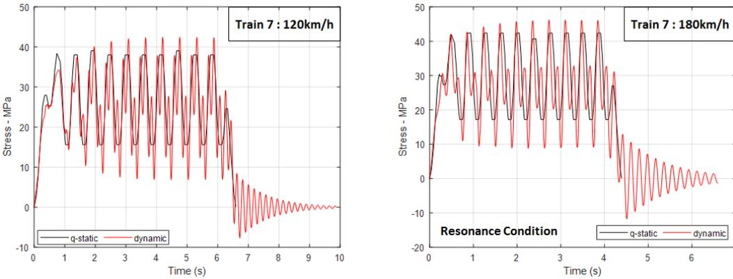
Figure 6. Bridge stress response at resonance conditions for Train 7.
