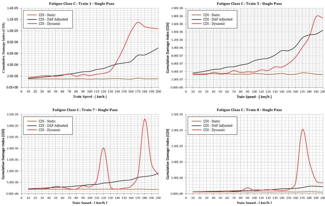
Figure 5. Bridge cumulative fatigue damage vs train speed for single train passages of 4 medium traffic trains.
