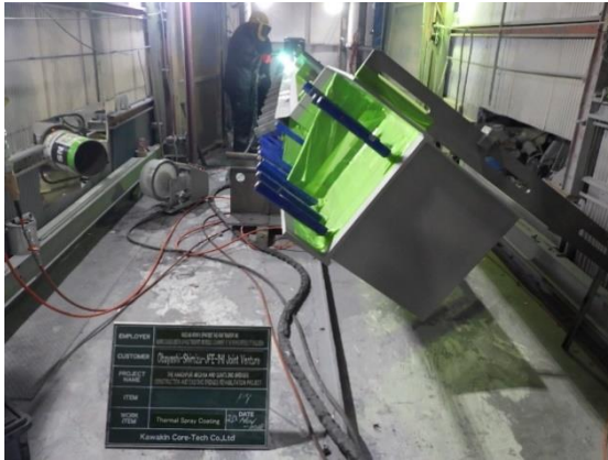
(a) Application of plasma arc thermal spray on the steel finger joints (b) After plasma arc thermal spray application Figure 17. Steel finger expansion joints with Al-Mg plasma arc thermal spray for the 2 nd Meghna, Gumti, and Kanchpur bridges
