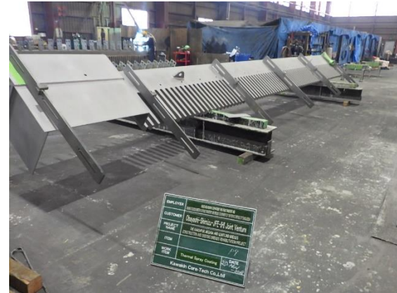
(a) Application of plasma arc thermal spray on the steel finger joints (b) After plasma arc thermal spray application Figure 17. Steel finger expansion joints with Al-Mg plasma arc thermal spray for the 2 nd Meghna, Gumti, and Kanchpur bridges
