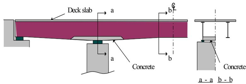
Fig. 5. Double composite girder bridge
