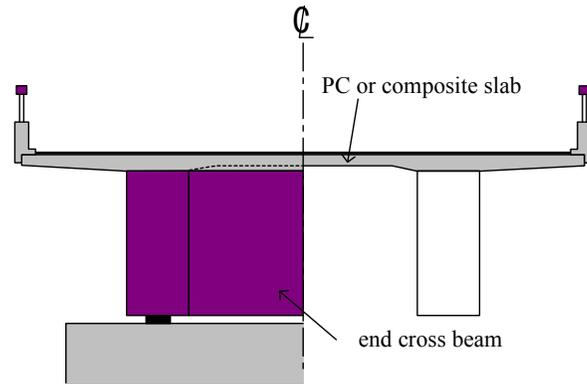
Fig. 2. Two-box girder bridge
