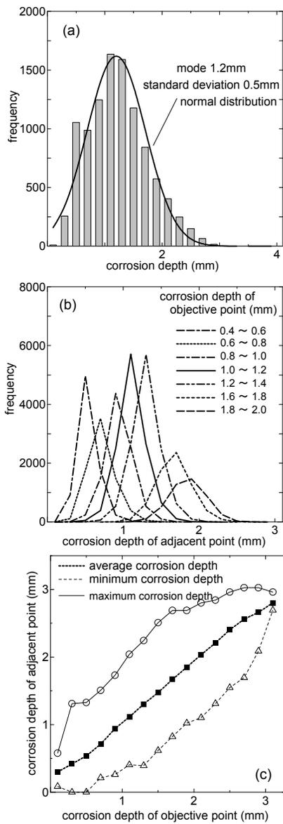
Fig.3. An example of measured results of corrosion depth in the B-bridge
