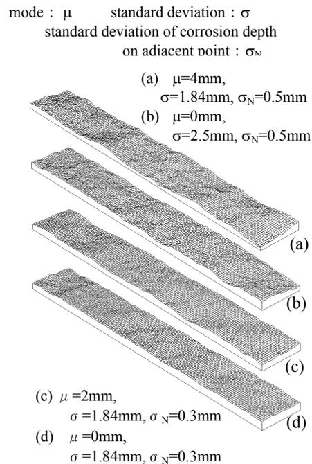
Fig.5. Examples of simulated corrosion surface
