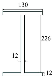
Fig.6. Cross section of beam
