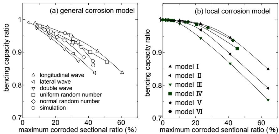
Fig.9. Bending capacity ratio arranged by maximum corroded sectional ratio
