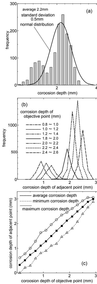
Fig.4. An example of measured results of corrosion depth in the C-bridge
