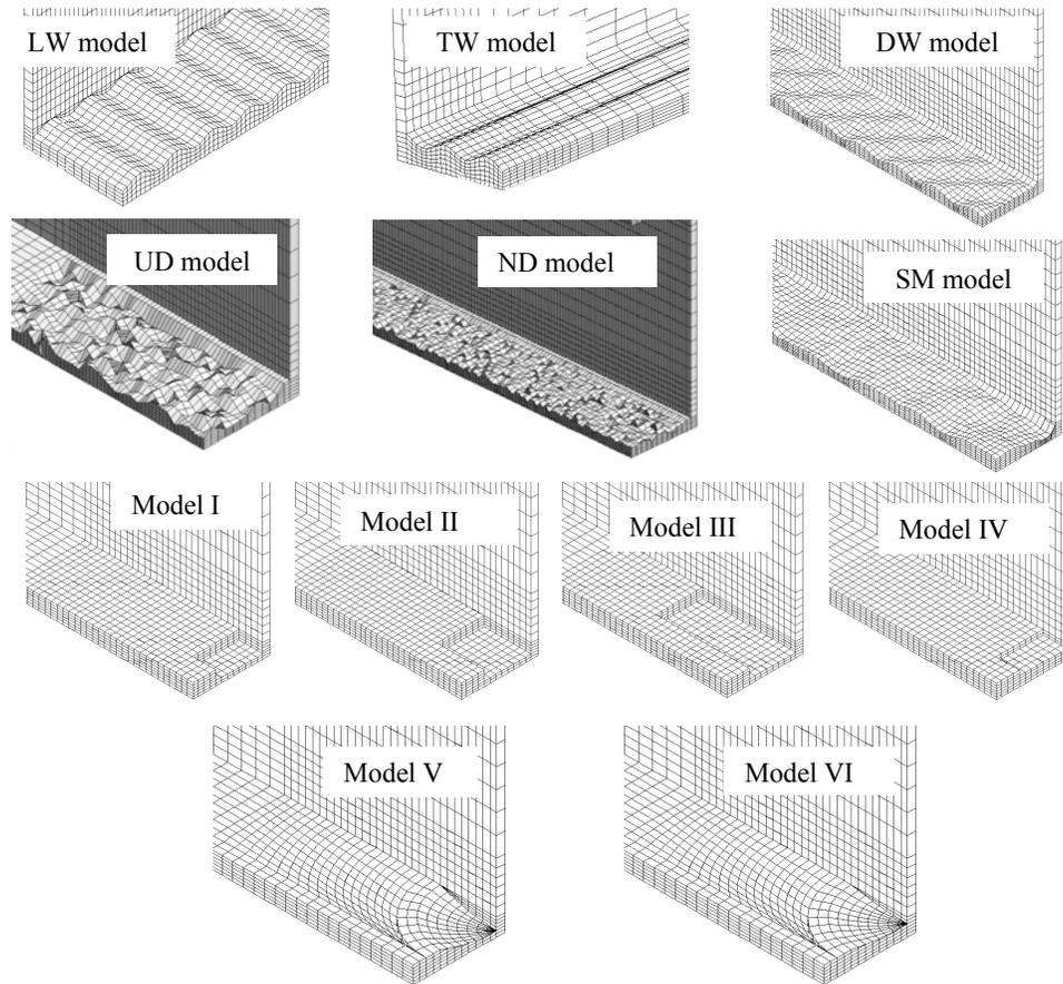
Fig.7. Finite element of each corrosion model
