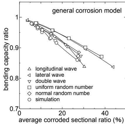
Fig.10 Bending capacity ratio arranged by average corroded sectional ratio
