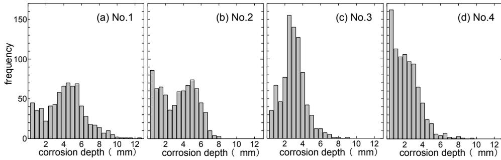
Fig.1. Distribution of corrosion depth on the upper flange of each girder (A-Bridge)
