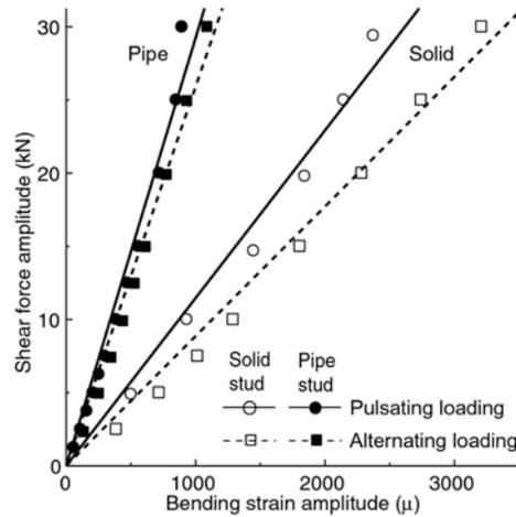
Fig. 10. Shear force amplitude-bending strain amplitude relation
