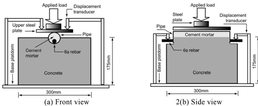
Fig. 2 Bearing test specimen
