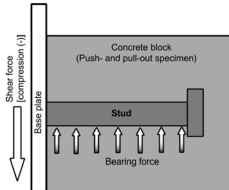
Fig. 3. Bearing force of concrete
