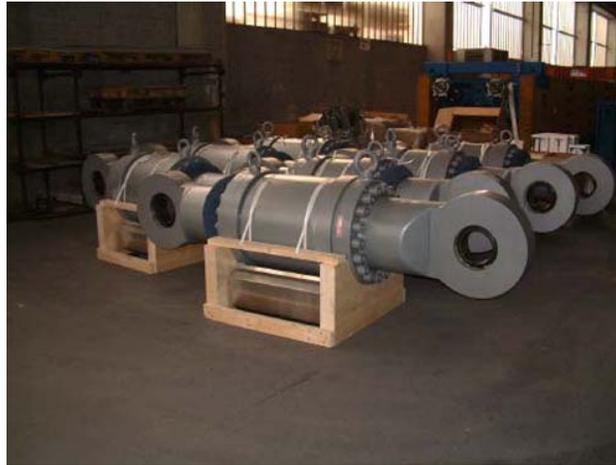
Fig. 13. View of STUs used in Paksey bridge
