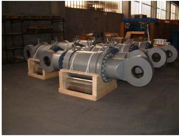
Fig. 13. View of STUs used in Paksey bridge
