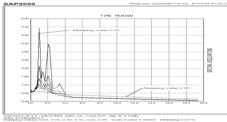
Fig. 11. Response spectrum curve (spectral accelerations vs time period)
