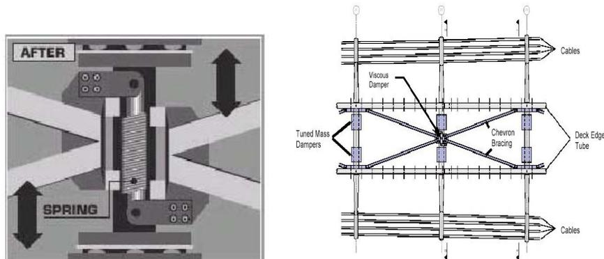
Fig. 2. Viscous and tuned mass dampers in The Millennium Bridge
