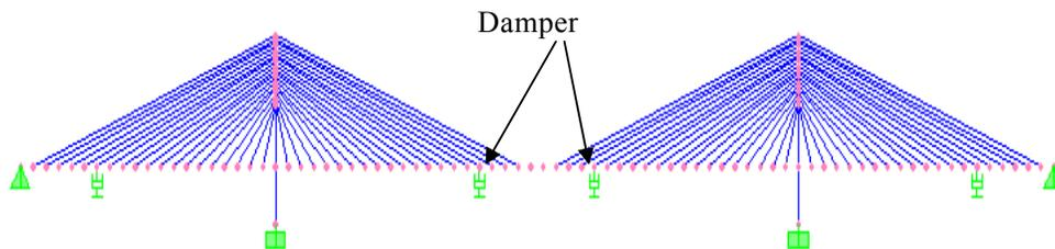
Fig. 6. Modeled cable-stayed bridge with damper
