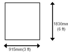
Figure 5.4 : Tower Bracing Cross Section
