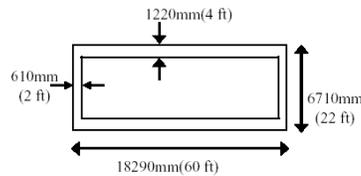
Figure 5.1 : Deck Cross Section
