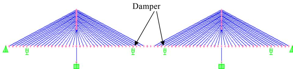
Fig. 6. Modeled cable-stayed bridge with damper
