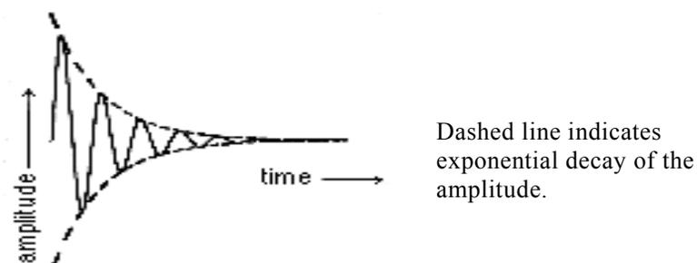
Fig .1. Exponential damping of a sine wave.
