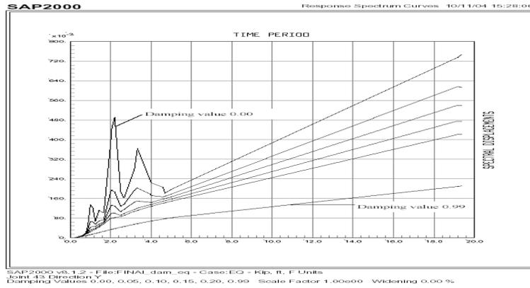
Fig. 9. Response spectrum curve (spectral displacements vs time period)
