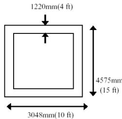
Figure 5.3 : Tower Cross-Section
