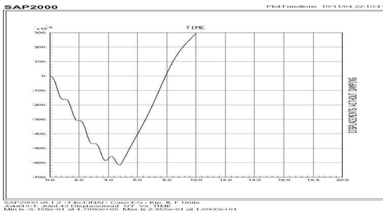
Fig. 13. Plot function analysis (displacements without damping vs time)
