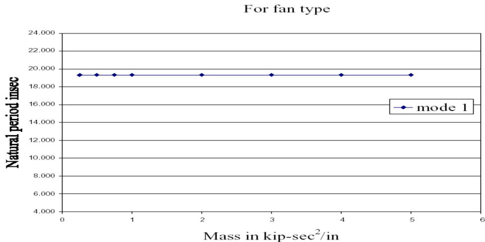
Fig. 8. Natural period vs mass of damper (for fan type)
