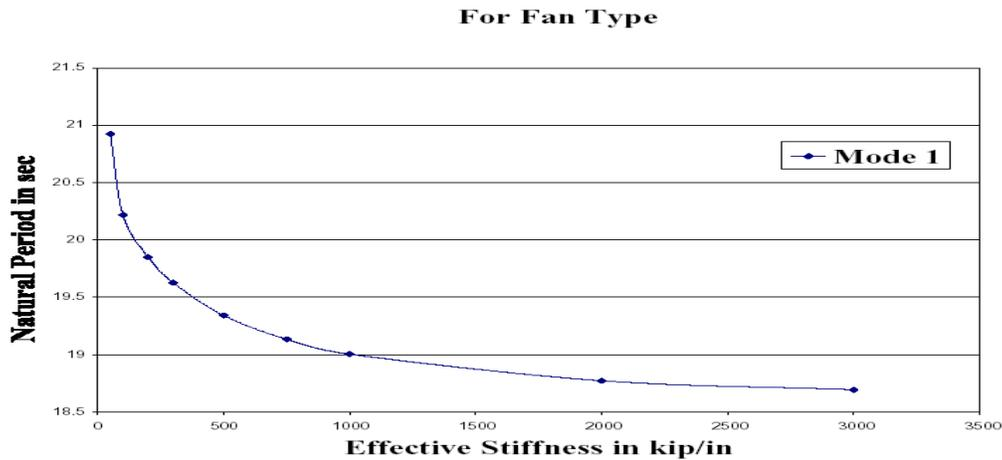
Fig. 7. Natural period vs effective stiffness of damper (for fan type)
