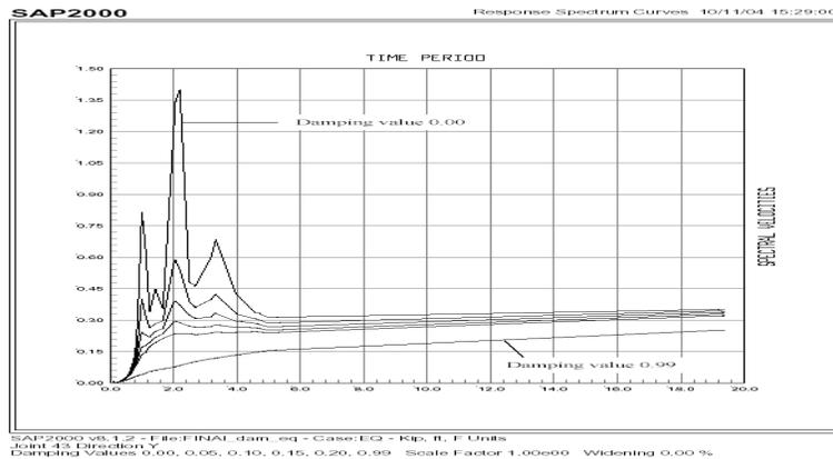
Fig.10. Response spectrum curve (spectral velocity vs time period)
