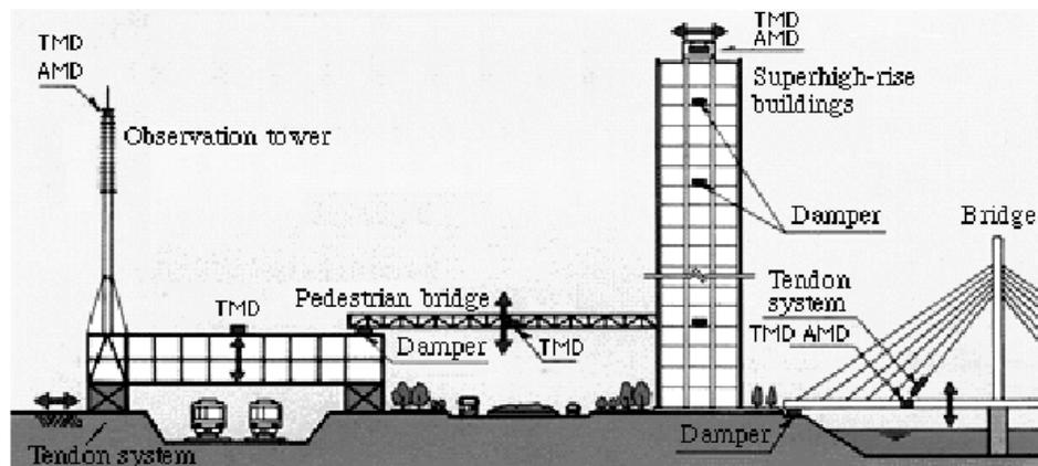
Fig. 4. A structural control device for earthquake-threatened structures
