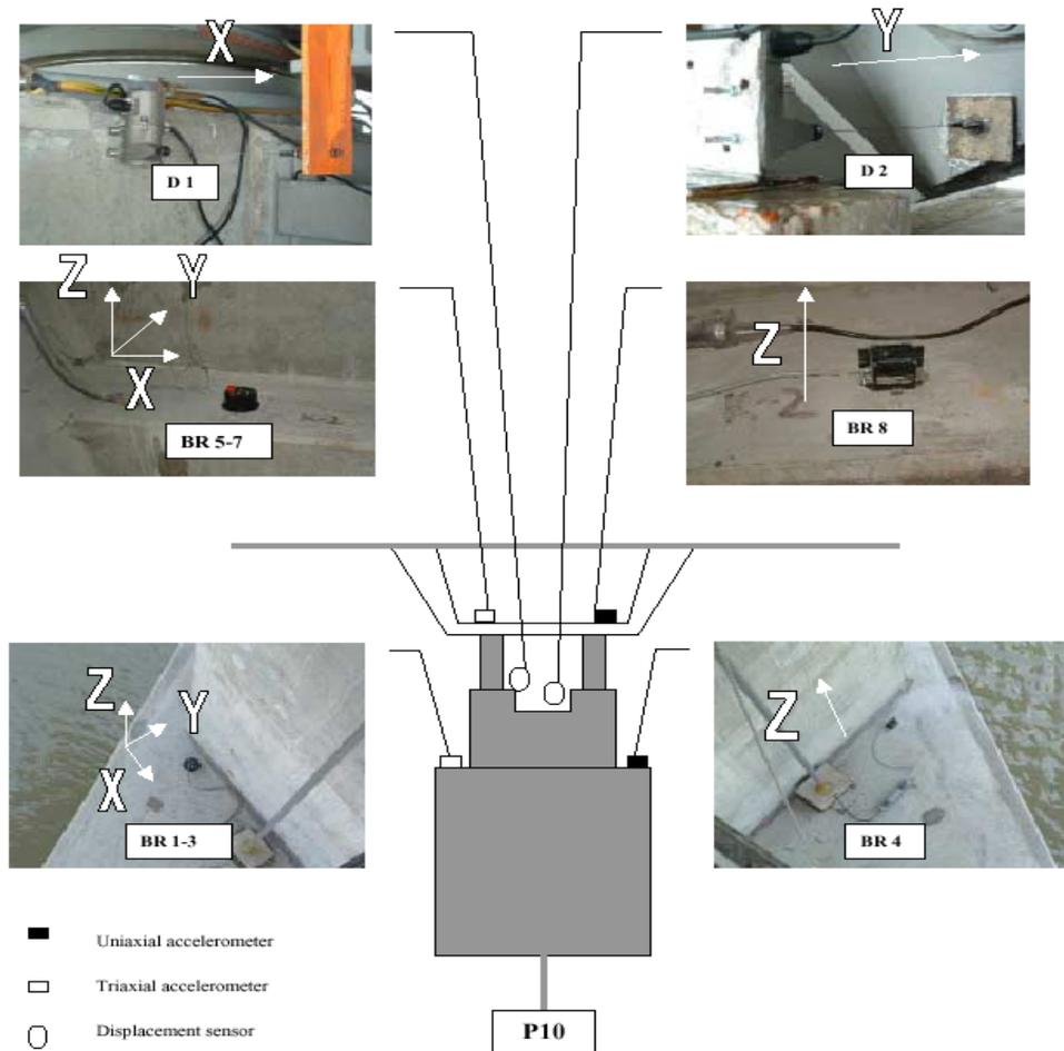
Fig. 6. Location of various accelerometer and displacement sensors at pile and pier.
