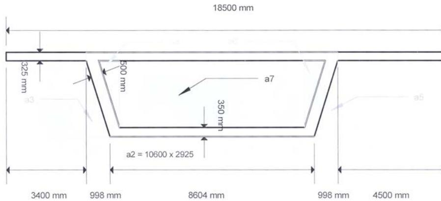
Fig. 13. Simplified deck cross-section at mid-span
