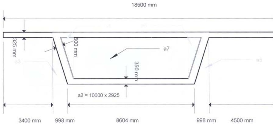
Fig. 13. Simplified deck cross-section at mid-span
