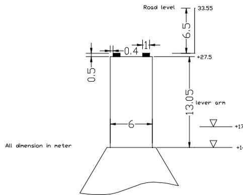
Fig. 4. Elevation of pier stem
