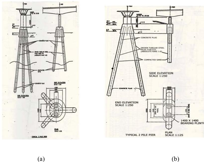
Fig. 2. General arrangement of piles (a) Three pile pier (b) Two pile pier
