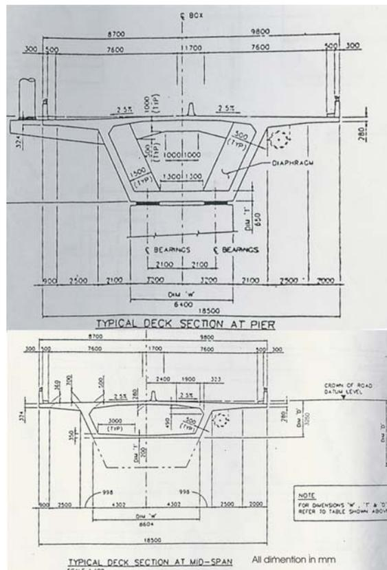
Fig. 5. Typical deck cross sections
