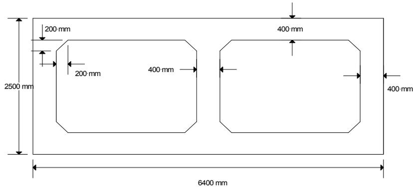
Fig. 3. Cross-section of pier stem
