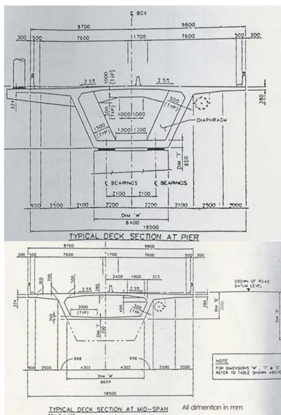
Fig. 5. Typical deck cross sections
